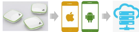
Figure 5. Bluetooth localization and tracking consisting of Bluetooth beacons, mobile app and cloud server (Source: SUTD)
