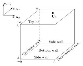
Fig. 3. Lid-driven cubical cavity. Geometry and definitions.
