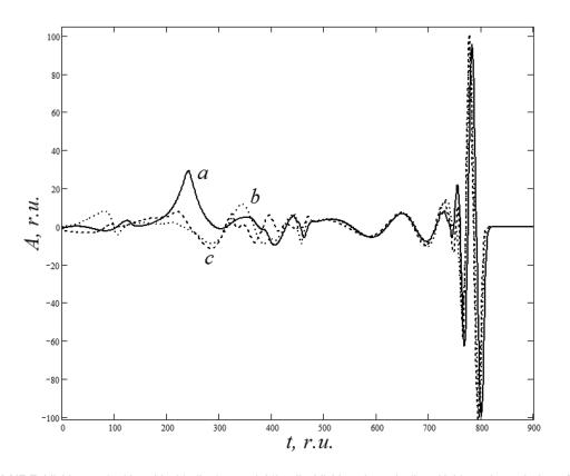
FIG. 3. Dependence of the vector potential on time for different values of the initial speed of pulse: (a) v/c = 0.93; (b) v/c = 0.95; and (c) v/c = 0.93. All quantities are given in relative units.
