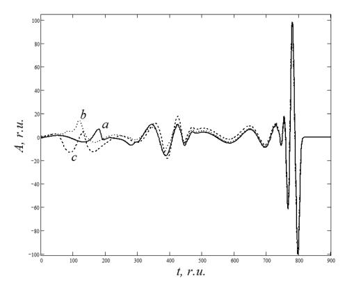
FIG. 4. Dependence of the vector potential on time for different values of the piezoelectric coefficient: (a) d=0.01; (b) d=0.05; and (c) d=0.1. All quantities are given in relative units.
