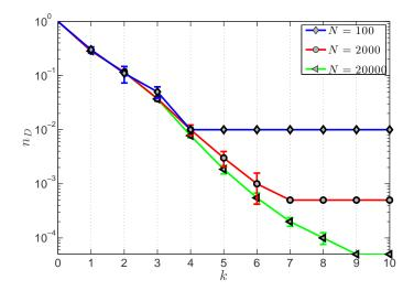
Figure 2: Density of required driver agents for a swarm with topologicallyinteracting members vs. the number of neighbors (k) for three different swarm populations (N). Results applying the exact controllability tool were collected for 10 distinct SSNs at each data point. The average density of driver nodes is calculated and the related standard deviations are illustrated by means of errorbars.
