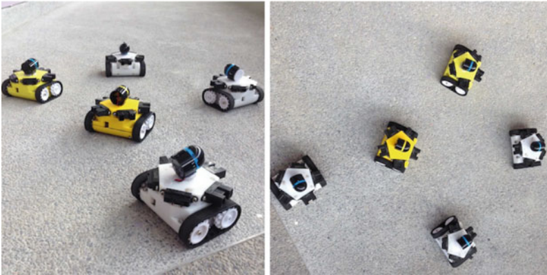
Fig. 1.1 Swarm of land robots “evobots” developed to perform collective surveillance. The bots exchange information about their respective localization, heading, and other sensed data using short-range communications through a mesh network. The distributed control algorithm is loaded onto each bot and collective computation is performed. Various collective behaviors such as heading consensus have been successfully implemented and tested. This swarm of evobots has been jointly developed with Prof. Erik Wilhelm at SUTD in the frame of the STARS project funded by the TL@SUTD
