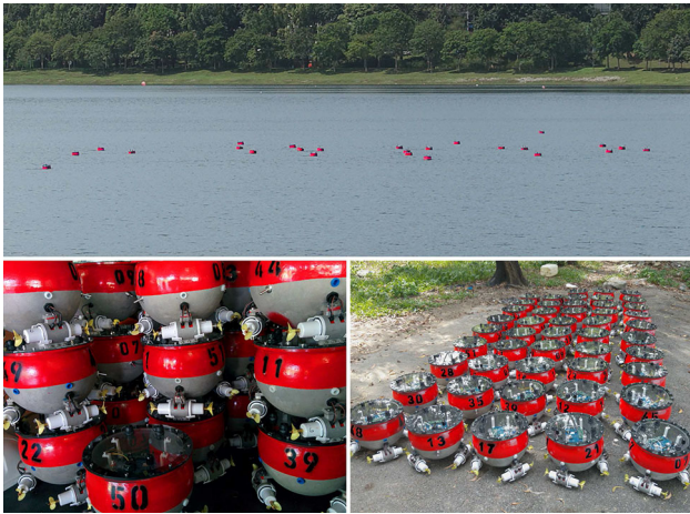
Fig. 1 A small fleet of autonomous surface vehicles. Top panel: 25 buoys of a BoB system collectively operating at Bedok Reservoir, Singapore. Bottom left: Buoys stacked up during transportation to the field site. Bottom right: 48 buoys lined up before deployment
