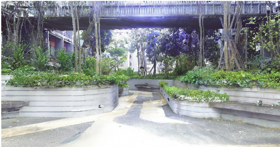
FIG. 12.2 Point cloud image of the Kampung Admiralty Level 4 Sky Garden. (Point cloud data was collected with FARO Focus 330D and visualized with FARO SCENE). No permission required .
