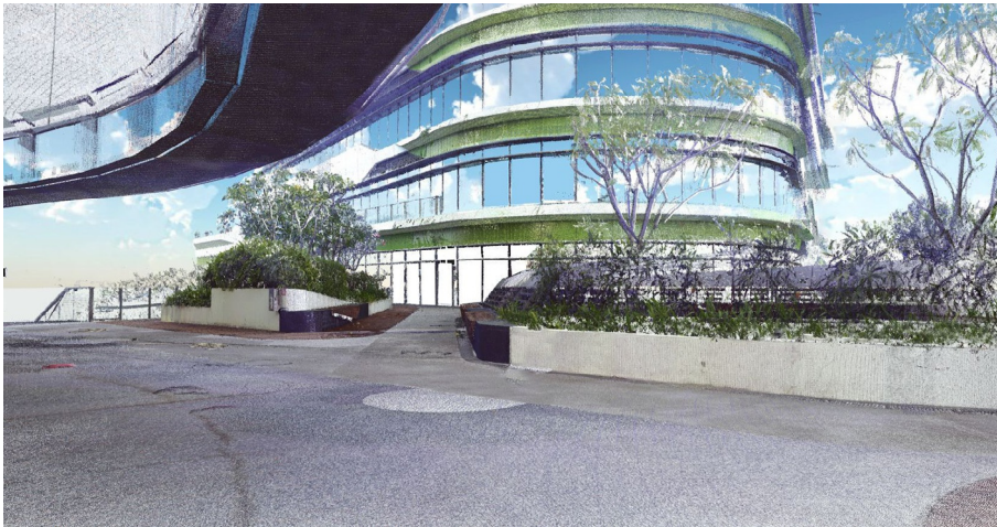
FIG. 12.4 Point cloud image of the SUTD Level 3 Sky Garden. (Point cloud data is collected with FARO Focus 330D and visualized with FARO SCENE). SUTD Cities: Urban Science and Design for Density.
