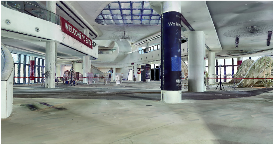
FIG. 12.3 Point cloud image of the SUTD Campus Center. (Point cloud data is collected with FARO Focus 330D and visualized with FARO SCENE). SUTD Cities: Urban Science and Design for Density.
