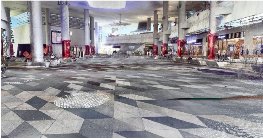
FIG. 12.1 Point cloud image of the Kampung Admiralty Level 1 Atrium. (Point cloud data was collected with FARO Focus 330D and visualized with FARO SCENE). SUTD Cities: Urban Science and Design for Density .
